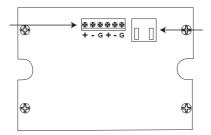
RJ45 connector for connection to the DZ-MATRIX. Maximum 100 meters of CAT 5E(or better) cable length.
