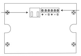
2 analog line outputs assigned to the RD 9/10 or 11/12 ports of the DZ-MATRIX
