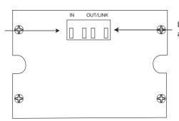
LINK RJ45 connection for additional remote controls
