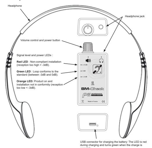
Note: The BM-Check is a magnetic field meter and approved by the EN60118-4 standard.
